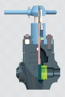
The Premium Oilfield Technologies Mud Gate Valve uses M2M<sup>™</sup> sealing technology. This technology allows our valve to be one of the longest lasting valves in the industry and is used in applications up to 7500 psi. Unlike conventional mud valves with rubber seats that wash out quickly, the NV-7500 uses single piece seat rings creating an upstream metal to metal seal. This upstream design helps eliminate debris contamination into the valve body and reduces wear on internal components.
